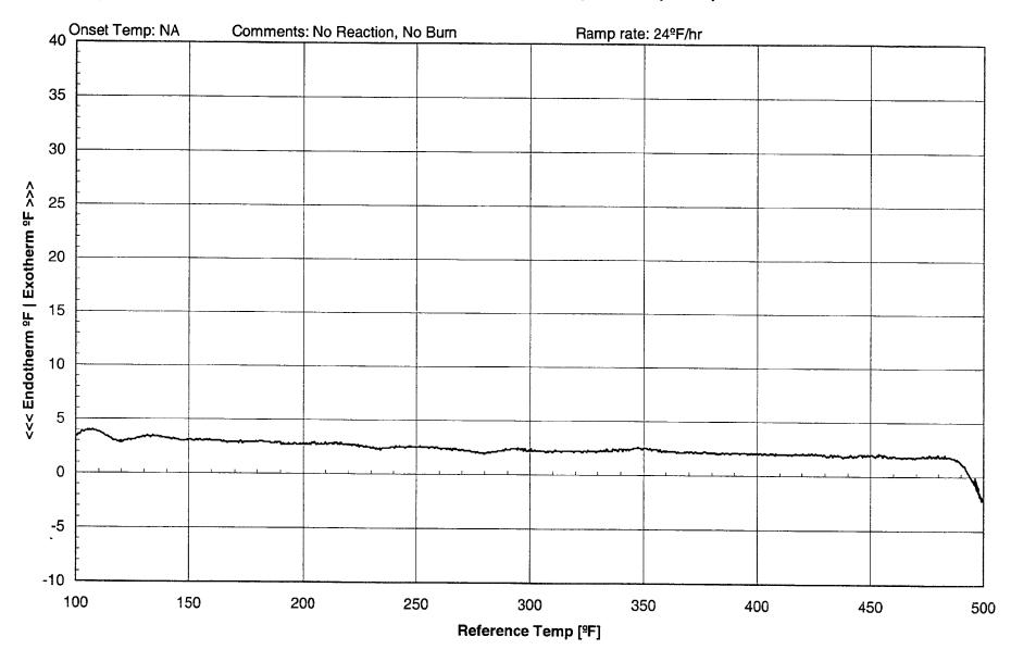
Figure A5: SBAT for 99/10 Sodium Chlorate/Sulfur Sample
