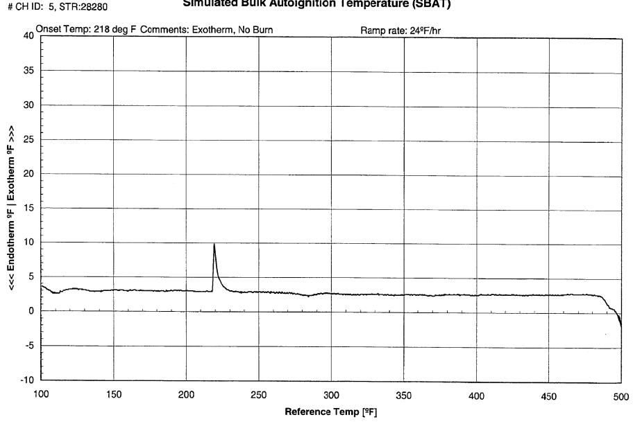
Figure A4: SBAT for 99.998/0.002 Sodium Chlorate/Oat Flour Sample
