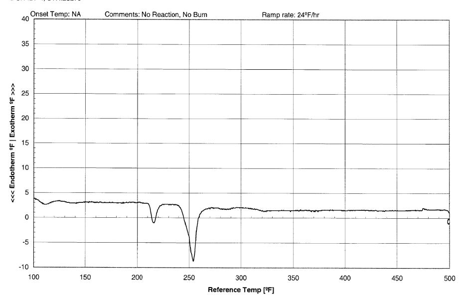
Figure A3: SBAT for 99.998/0.002 Sodium Chlorate/Sulfur Sample
