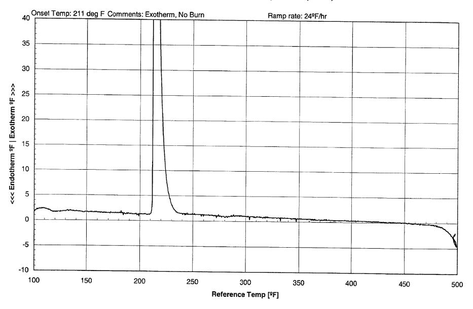
Figure A6: SBAT for 99/10 Sodium Chlorate/Oat Flour Sample
