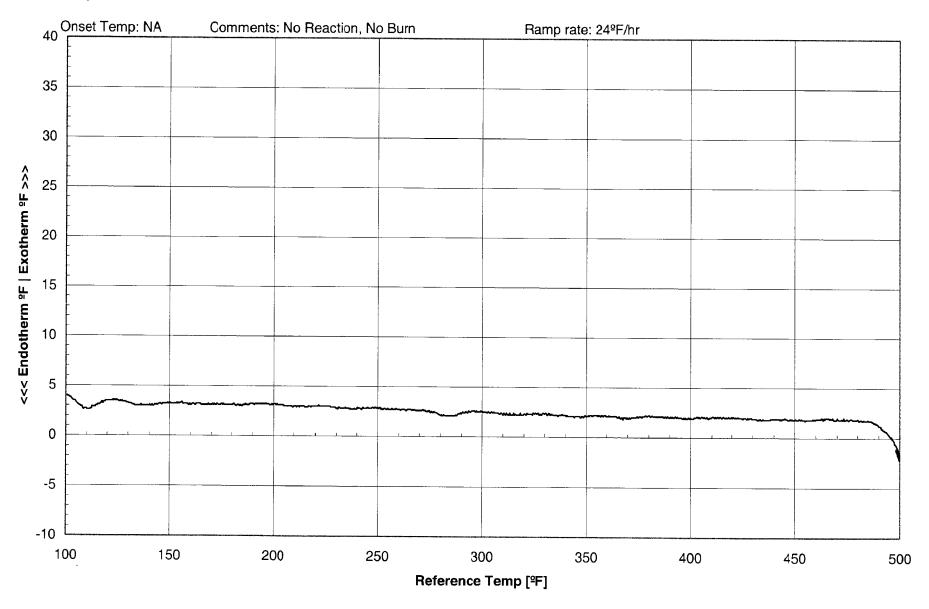
Figure A2: SBAT for Sulfur Sample
