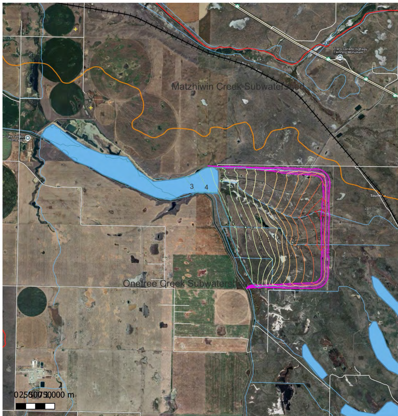
Figure 12: Impact of the Reservoir Expansion at Maximum Capacity Over 90 Days
