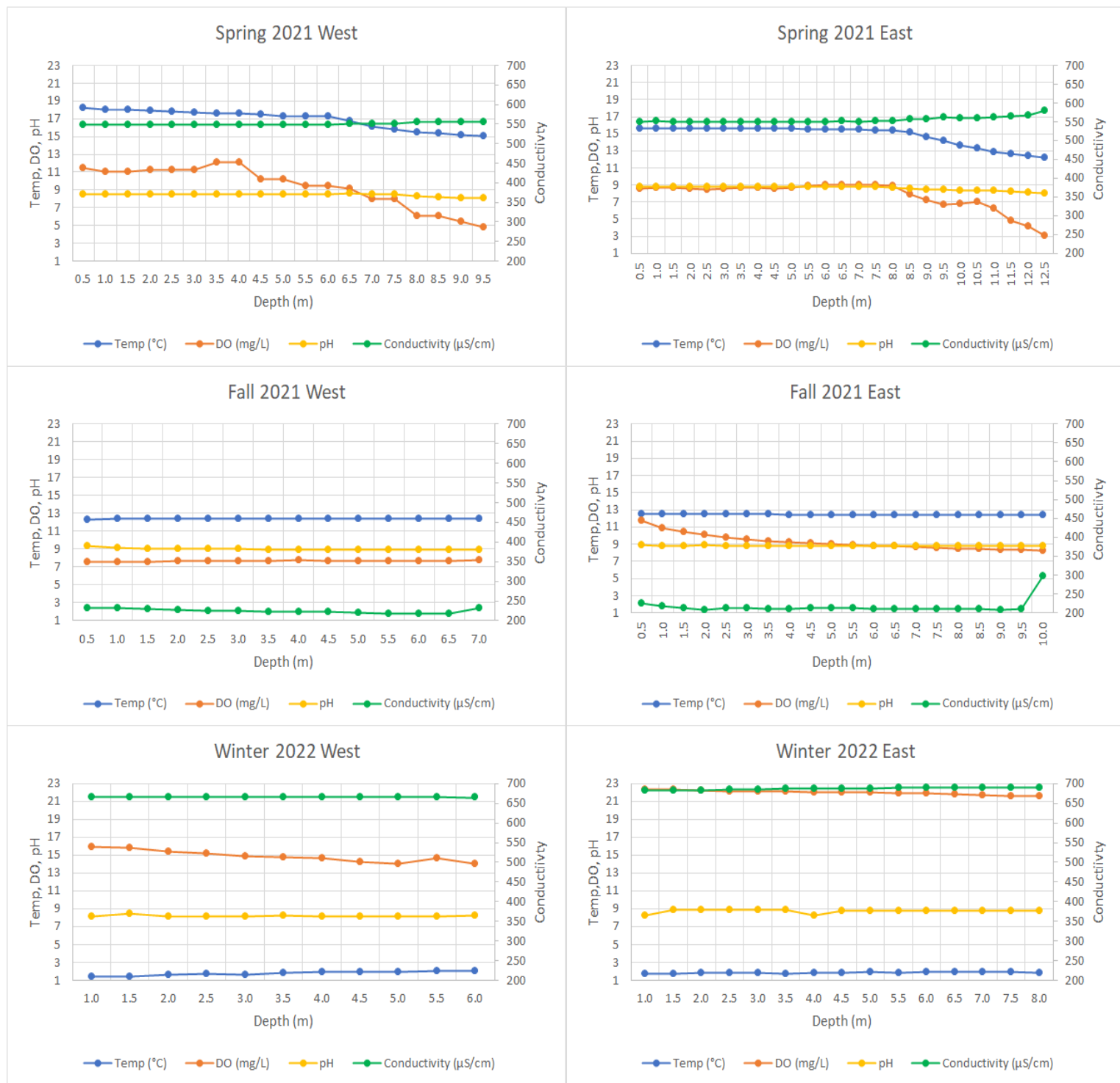
Figure F1-7: Water Quality Parameters Sampled at Snake Lake Reservoir 2021-2022
