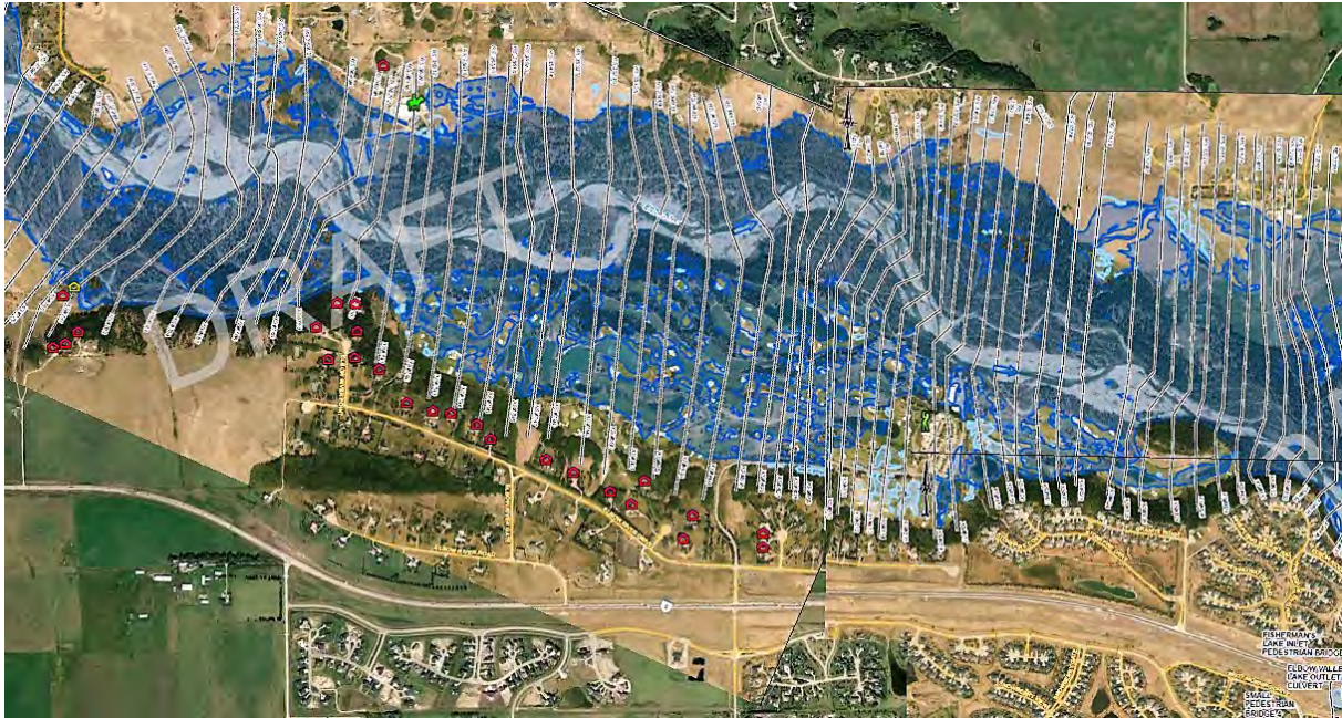
Figure 8 Residence and GLENCO Golf Course Fairways at Risk of Flooding (1:50 yr.)
