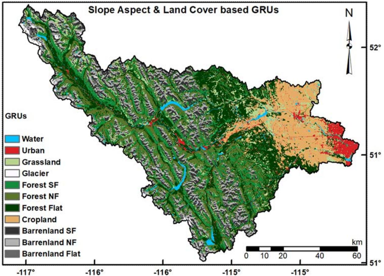
Figure 5. Grouped Response Unit discretization by combining slope aspect and landcover
