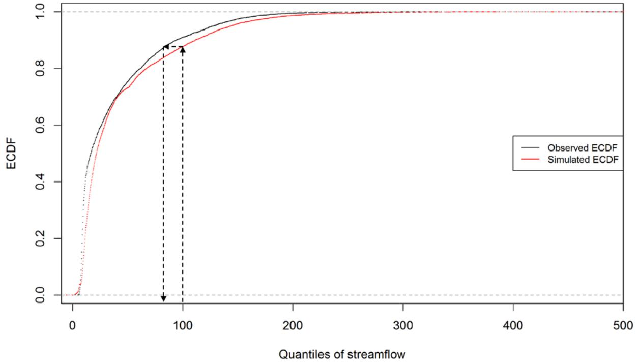
Figure 10. A schematic of the quantile mapping (QM) method for Bow River Basin at Banff.
