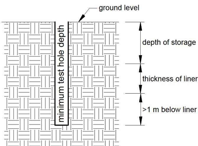
Figure 1. Determining minimum test hole depth for a proposed compacted soil liner.
