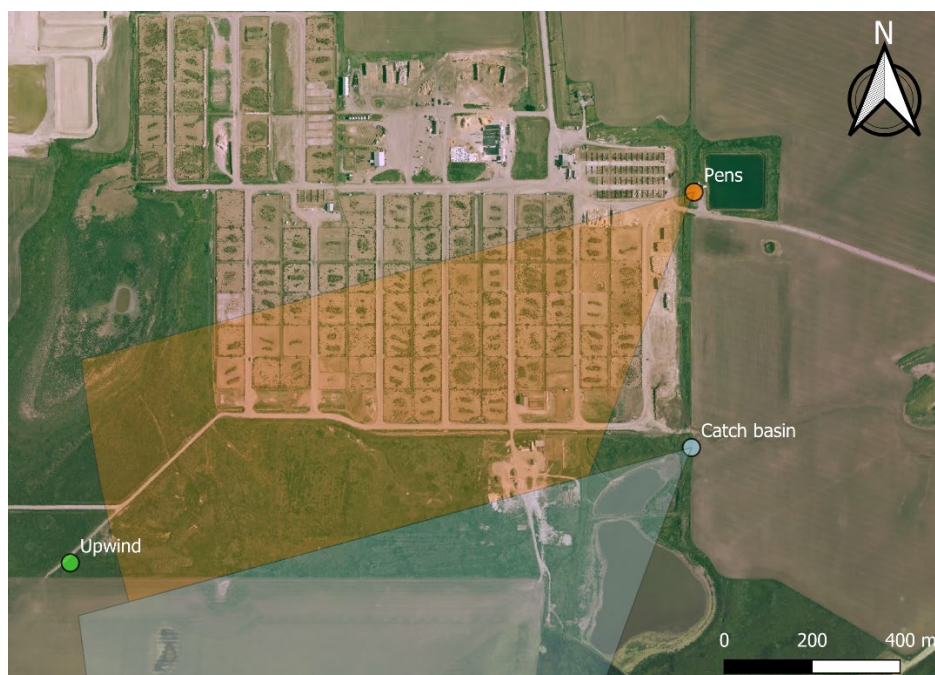
Figure 1 Location of the air monitoring stations at Rimrock Cattle Company Ltd. targeting the feedlot pens and catch basin features. Air quality was analyzed for wind directions ranging between 210° and 260°, shown by the coloured buffers.
